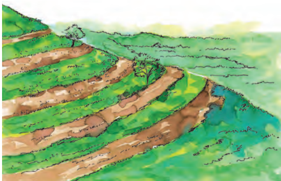
Continuous contour trenches (CCT)
