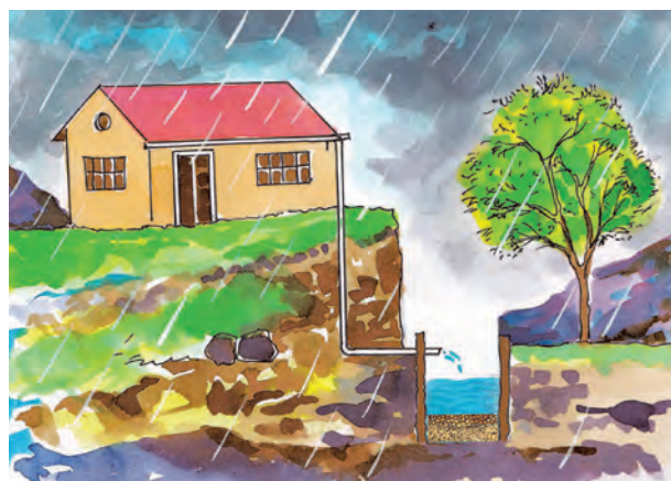
Making rainwater seep into the soil
